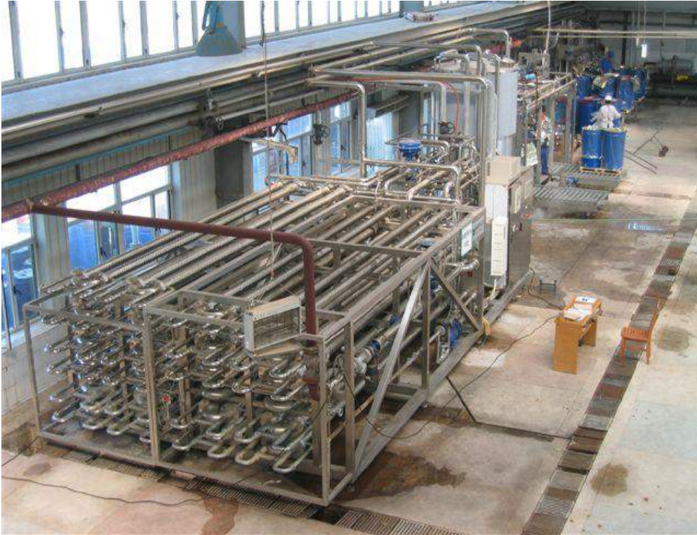
Tube in tube sterilizer
