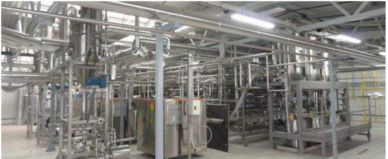
Tube in tube sterilizer
