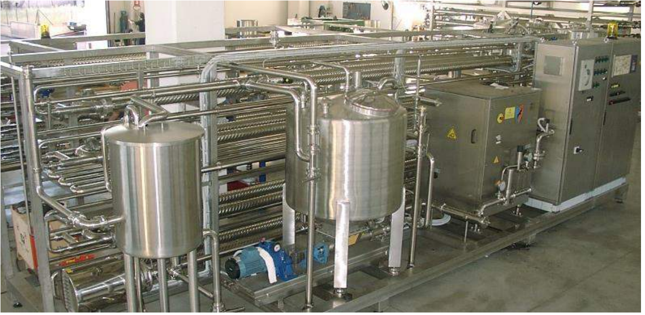
Tube in tube sterilizer
