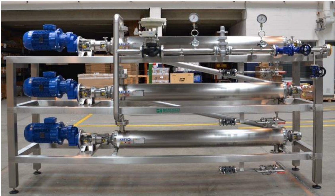
Scraped surface heat exchanger
